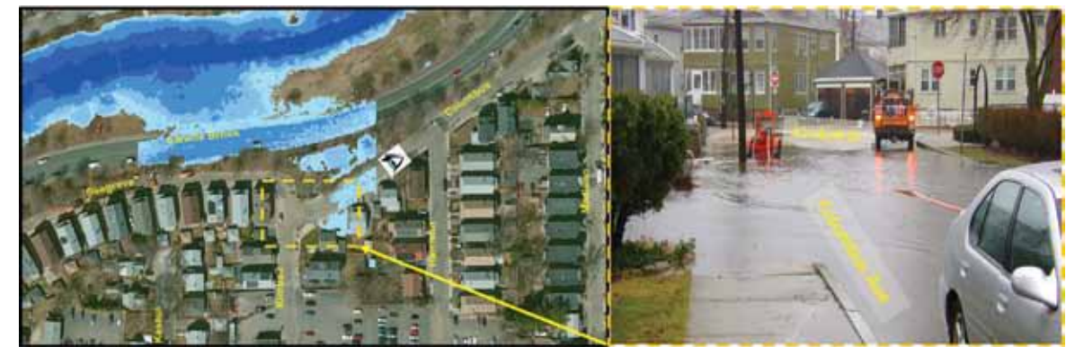
Figure 12. Comparison between observed and simulated street flooding at Kimball Street and Columbus Avenue during the March 2010 storm
