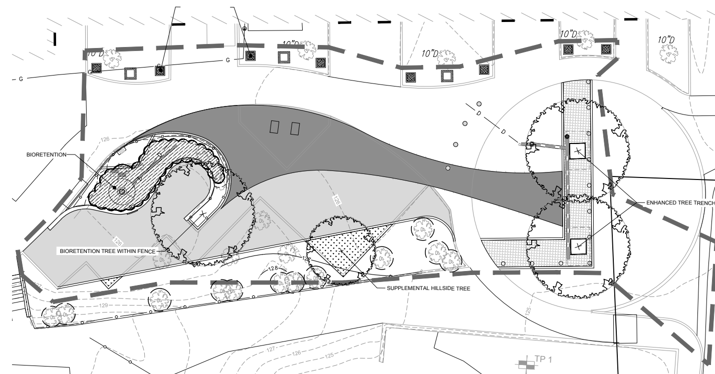
Stormwater tree pits were used to separate the play yard at the David A. Ellis Elementary School from the pick-up/drop-off area and other vehicle traffic from the adjacent Museum of the National Center of Afro-American Artists
