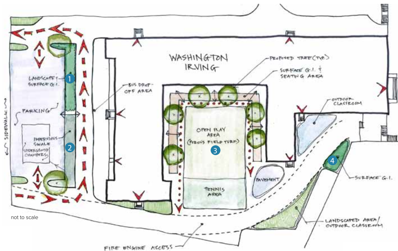
Washington Irving Middle School conceptual plan: 1. Bioswale 2. Concrete swale 3. Open play area with field turf and porous pavers and trees 4. Bioretention
