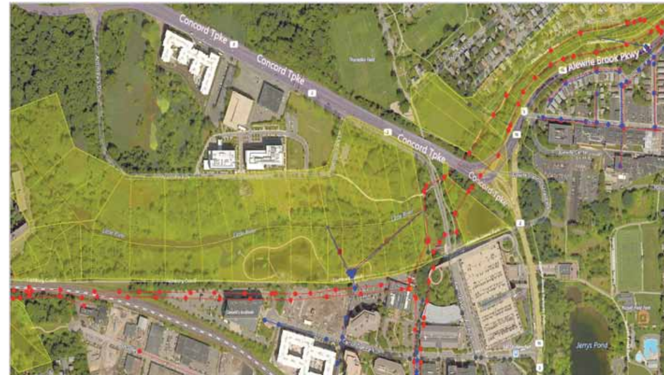
Figure 6. Sewer and river interconnectivity along Alewife Brook. The yellow tinted area represents the river reach; the transverse dotted lines are river cross-sections; and the red, blue, and green circles and lines represent the sanitary, storm, and combined sewer manholes and sewers, respectively.
