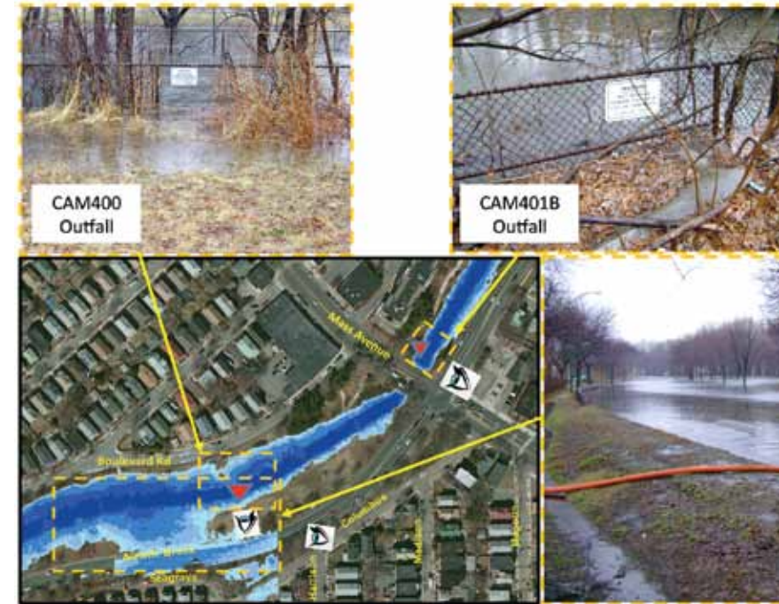
Figure 11. Comparison between observed and simulated flooding along Alewife Brook Parkway during the March 2010 storm
